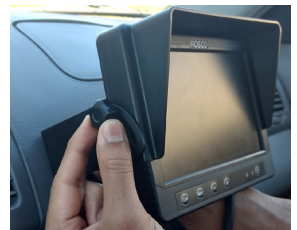
Attaching monitor to U bracket using thumb screw
