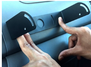
Attaching U bracket to vehicle.
