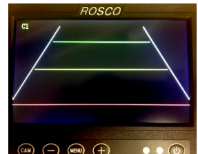
Appearance of the Backup Grid
