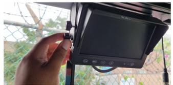
Attaching monitor to U bracket using thumb screw
