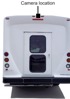
Mount the camera high and centered on the rear of the vehicle.
