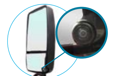
REAR LOOKING CAMERA
