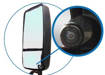
REAR LOOKING CAMERA
